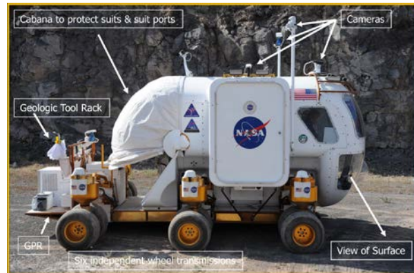
Fig. 1. A GPR unit installed beneath the aft deck of an LER.
