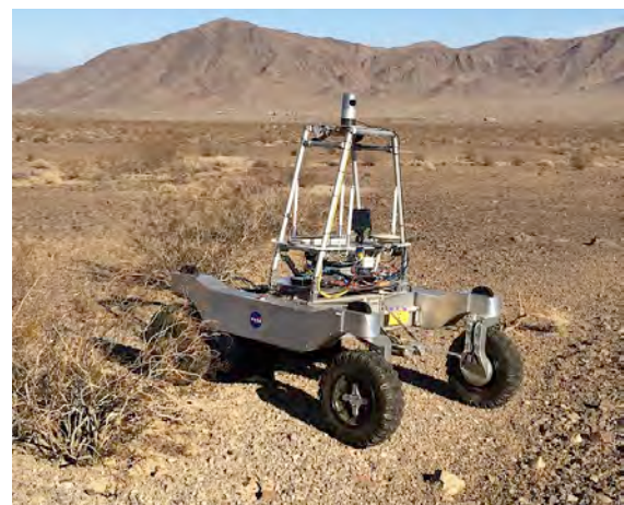
Fig. 2. KREX-2 rover traversing desert pavements and nearby features during the MVP test. The neutron spectrometer is mounted between the two wheels on the right.
