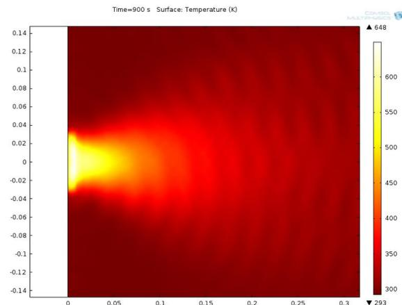
**Fig. 2** – Multiphysics simulation (COMSOL) of 2.4 GHz Microwave propagation into Lunar simulant.
