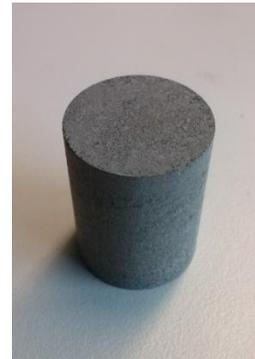
**Fig. 1** – Processed DNA sintered simulant via conventional resistive heating oven (vacuum).
