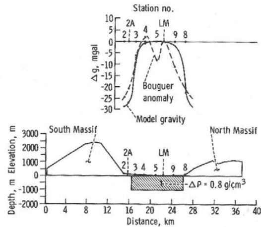
**Figure 2:** The Apollo 17 Lunar Traverse Gravimeter was used to infer the presence of a  $1\text{ km}$  thick basalt block beneath the Taurus-Littrow valley floor [1].
