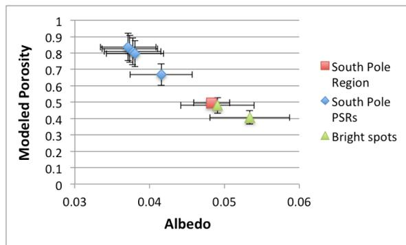
**Figure 2: LAMP Lyman- $\alpha$  albedo and modeled porosity. Error bars for the albedo are based on counting statistics, which are then propagated to the modeled porosity value.**
