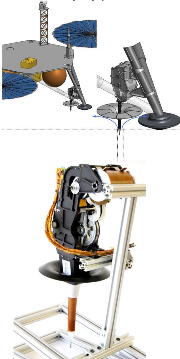
Figure 3. Pneumatic heat flow probe uses compressed helium gas to advance below the regolith surface.
