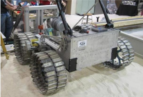
**Figure 3: Metallic compliant wheel**
