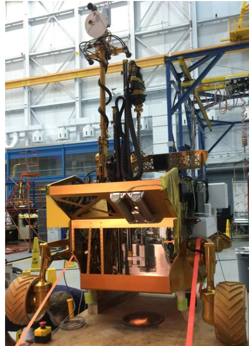
Figure 4. Lunar Resource Prospector Drill mounted on the NASA JSC rover.
