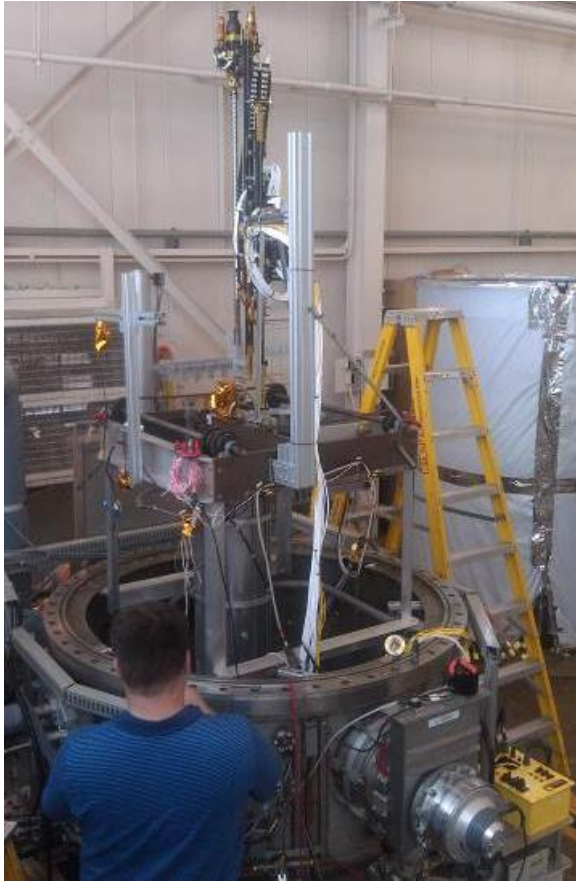
Figure 3. Lunar Resource Prospector Drill mounted inside VF13 lunar chamber facility at NASA Glenn Research Center.
