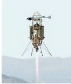
Figure 3: Griffin's precision landing and hazard avoidance system in a test flight on Masten's Xombie
