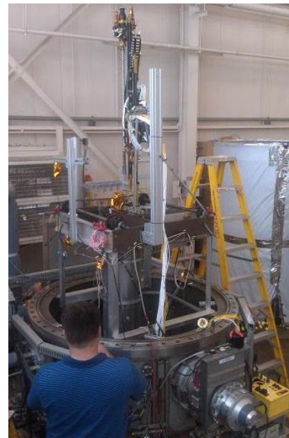
Figure 3. Lunar Prospecting Drill mounted inside VF13 lunar chamber facility at NASA Glenn Research Center.
