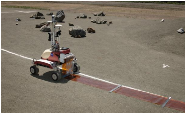
Figure 1. Deployment of Kapton film by crew aboard the ISS using the teleoperated K10 rover at the NASA/Ames Roverscape.
