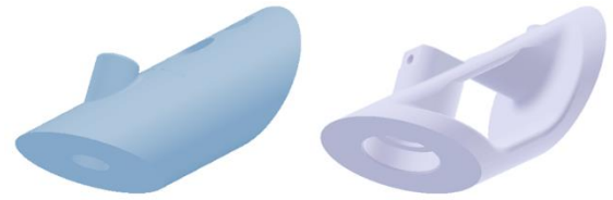
Figure 6: Comparison of the links of the CubeSat robot. Left: the original link form. Right the optimized weight and material requirements form.
