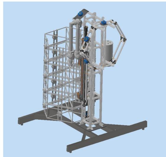
Figure 5: CAD visualization of dLSAFFE. In the back, the SMTs in their storage location can be seen.
