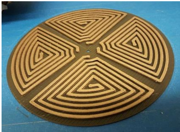
Figure 4: Fully 3D printed armature made from the conductive copper filament.
