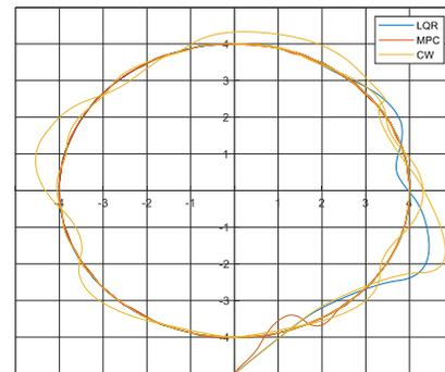
Figure 3: Comparison of the Fly around Orbits with Three Controllers
