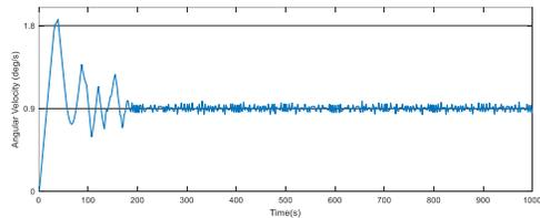
Figure 8. LQR- Change in Angular Velocity with Time
