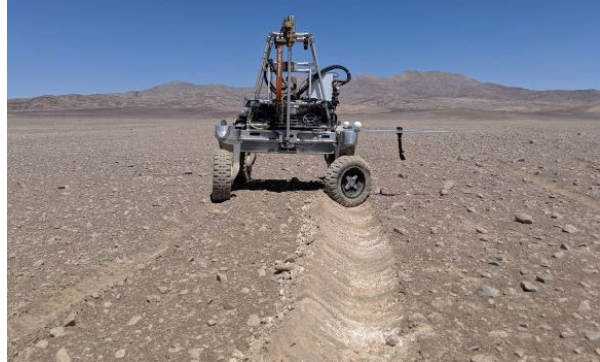
Figure 1. KREX-2 rover in the Atacama Desert with a trench dug by a wheel at 60°.
