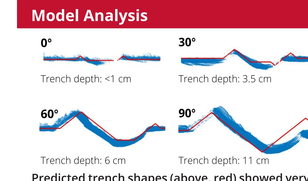
Predicted trench shapes (above, red) showed very good qualitative agreement with those measured in the Atacama (above, blue). Scans were manually centered, and wheel sinkage was manually extracted from LIDAR data, though it can also be predicted to some degree with terramechanics models. As previous tests in [2] were on prepared, uniform substrate, this was the first demonstration in a real-world environment.
