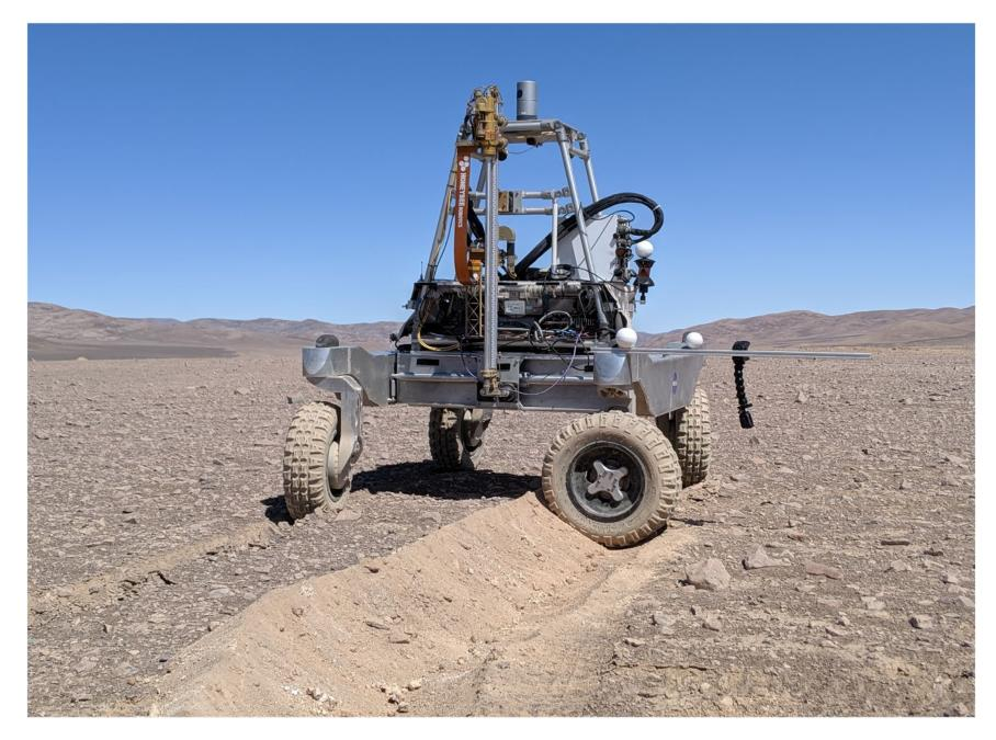
The wheels of planetary exploration rovers can be used to modify terrain through careful choice of wheel **speed and angle**, in what we call Nonprehensile Terrain Manipulation (NPTM). This has been done in an ad-hoc manner by Mars rovers [1]. Previous work predicting the shape of terrain left behind a rover wheel while has been validated in a controlled laboratory setting [2].
