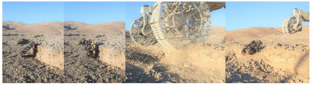
A robot-teaming scenario was conducted with KREX-2 and the MiniRHex [3] platform (above). MiniRHex attempted to ascend a body-scale step in the terrain (left), but was unable to and flipped over (center left). **KREX-2 used its wheel to** dig a ramp into the terrain (center right), which MiniRHex was able to ascend (right).
