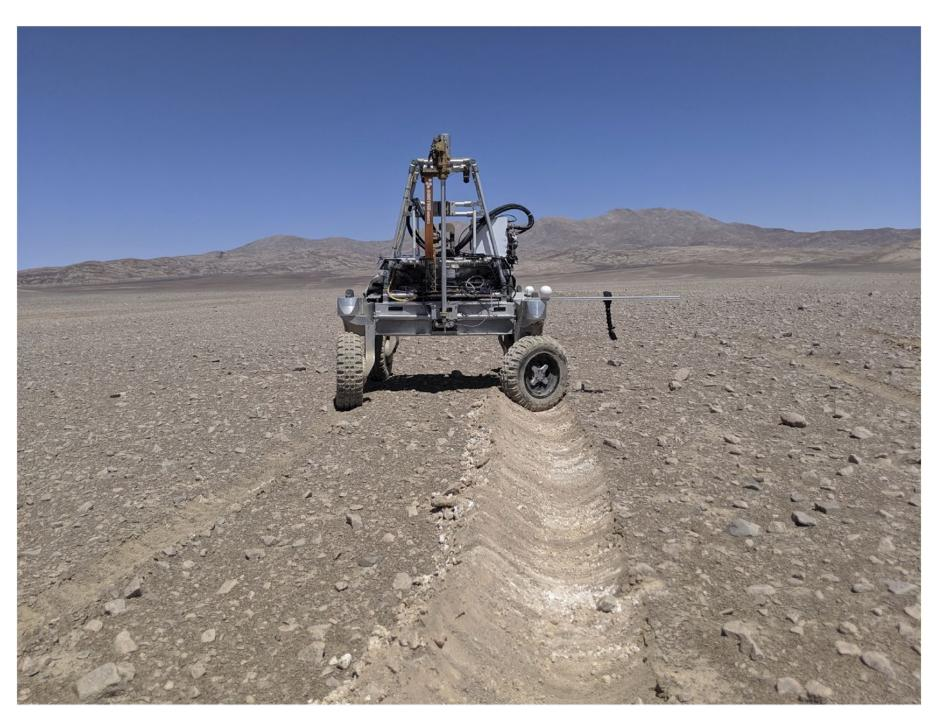
Hand-tuned trenching primitives were run with the rover driving at 20 cm/s, with the rear right wheel spinning at 50 cm/s and at 0°, 30°, 60°, and 90° angles relative to rover direction of travel.
