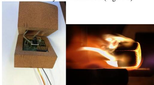
**Figure 2: Thermal Plug/Pressure Test with Ablative TPS at Plasmatron.**
