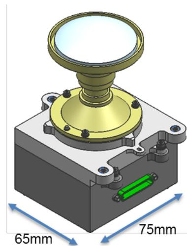
*Figure 1. The basic EECAM design consists of a fixed focus lens mounted to a sensor head. Pictured above is the Mars 2020 Navcam camera.*
