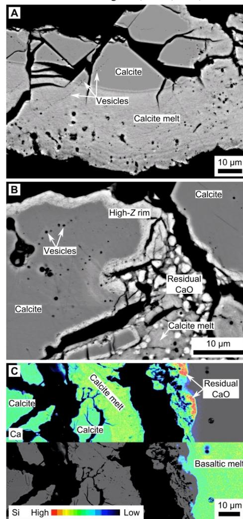
**Fig. 1** Melting of calcite (a), degassing of calcite (b), and distribution of Ca and Si among the calcite melt zone (c).
