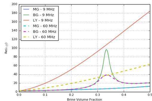
**Fig 1.** Real part of the complex permittivity for a mixture containing 50% ice with varying volume fractions of liquid brine and vacuum pores, using the Maxwell Garnett (MG), Polder-van Santen or Bruggeman (BG), and Looyenga (LY) mixing approaches.
