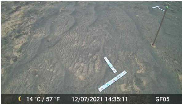
Figure 4: Image acquired from one of the time-lapse cameras showing the use of scales during the acquisition of high-quality images for use in shape from shading. The vertically positioned rod is used to define the z-axis when processing the images.
