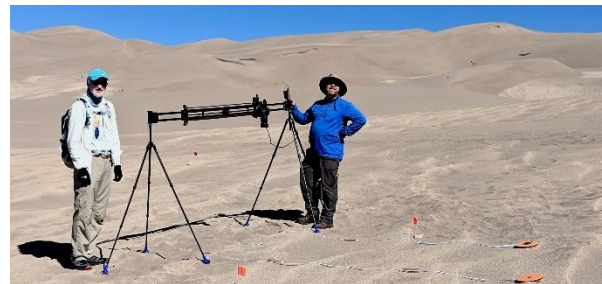
Figure 1. A field macro stereophotogrammetry rig.
