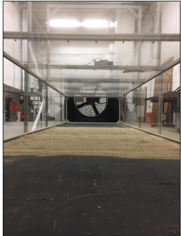
Figure 2: Wind tunnel experimental setup showing 7 x 1.7 x 1 m dimensions, fixed-point Kinect station visible at top. Sub-mm scale grains are readily mobilized by wind speeds > 8 \text{ m/s} , creating saltation impacts across the tunnel floor.
