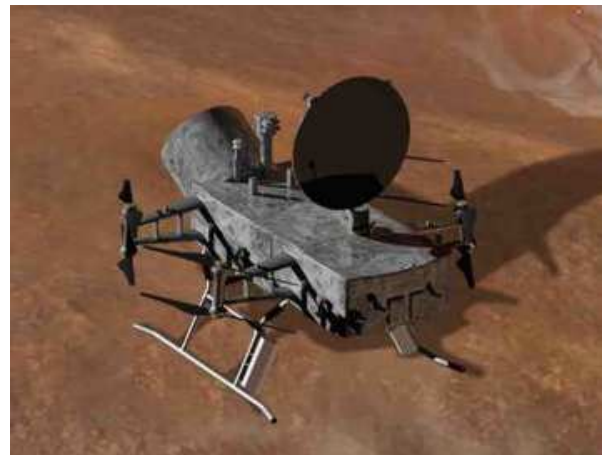
Fig. 2. Artist's impression of the Dragonfly relocatable lander. Outboard rotors allow the controlled application of wind stress to surface materials.
