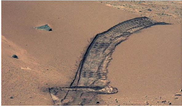
Fig. 5. Portion of MastCam image, sol 538. Rover wheels did not sink more than a few cm when traversing the TAR. Dark sand exposed in tracks.
