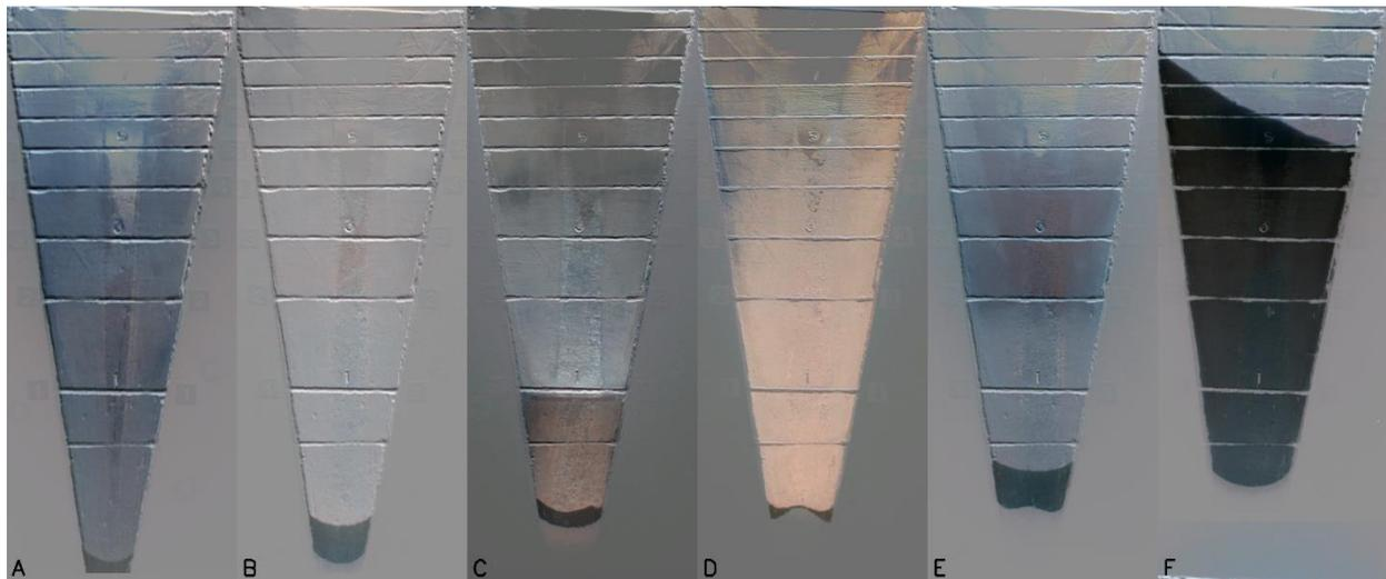
**Figure 2:** Volume results from the Mars Experimental BSNE. The images are the difference between an image acquired just prior to a sediment flux event and an image acquired after the event. The lines indicate volume from bottom to top: 50 cc, 100 cc, 200 cc, 300 cc, etc. (A) (B) (C) Precipitation (D) (E) (F) Large nighttime event.
