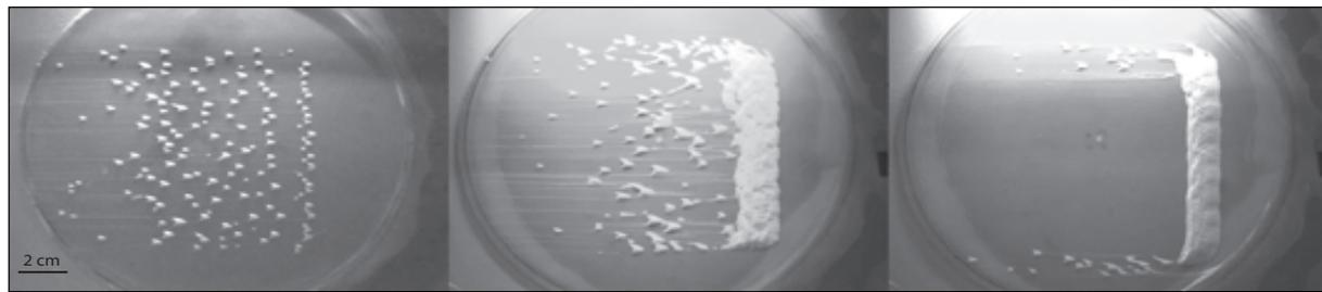
Figure 2: Dune field morphologies under unidirectional wind depending on sand supply – Right to left: low sand availability ( $Q_{in} 0.017\text{mm}^2/\text{T}$ , barchans fields), medium availability ( $Q_{in} 0.11\text{mm}^2/\text{T}$ , barchnoid ridge), high sand availability ( $Q_{in} 0.24\text{mm}^2/\text{T}$ , transverse dune)
