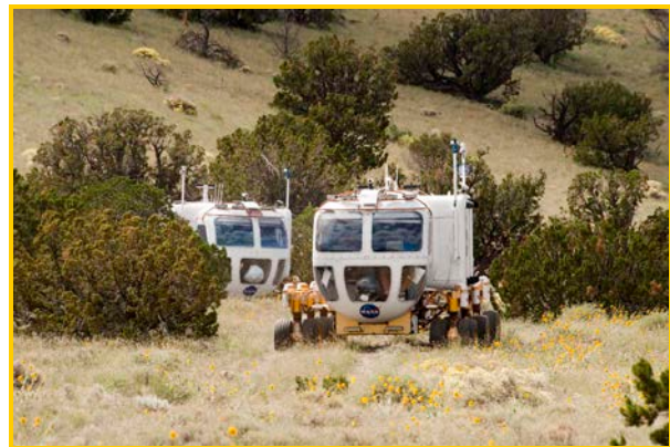
Fig. 2. Dual LER in a simulation of a lunar mission involving a crew of 4 (2 in each vehicle).
