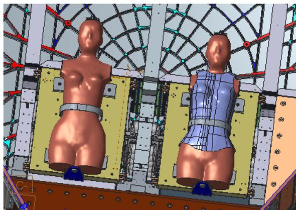
**Figure 1. MARE configuration as baselined for Orion consists of two radiotherapy phantoms located at seat positions 3 and 4 in the spacecraft. The phantom at position 4 is fitted with the AstroRad astronaut radiation shield.**
