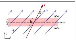
Figure 1: Schematic diagram of wave propagation in an active region. This illustrates the scenario of a wave with wave vector  $\mathbf{k}$  approaching a magnetic region from below. Here a is the Alfven velocity, c is the sound speed, k makes an angle  $\alpha$  to the magnetic field  $\mathbf{B}$ , which itself makes an angle  $\theta$  to the vertical at a=c layer. Adapted from [5].
