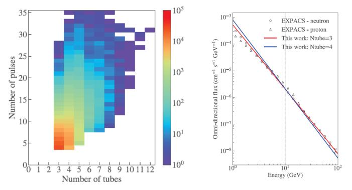
The total number of neutrons detected and the number of adjacent detectors hit vary with incident energy. Their distribution (left) can be used to determine the particle spectrum (right)
