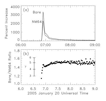
South Pole station has both standard neutron monitor and an array of "bare" detectors lacking the lead producer.
