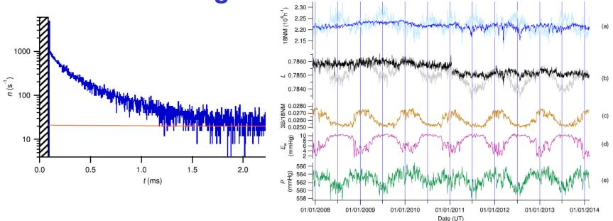
The distribution of intervals between successive neutron detections (right) can be calibrated to yield the spectral index of the cosmic rays (black trace, right).
