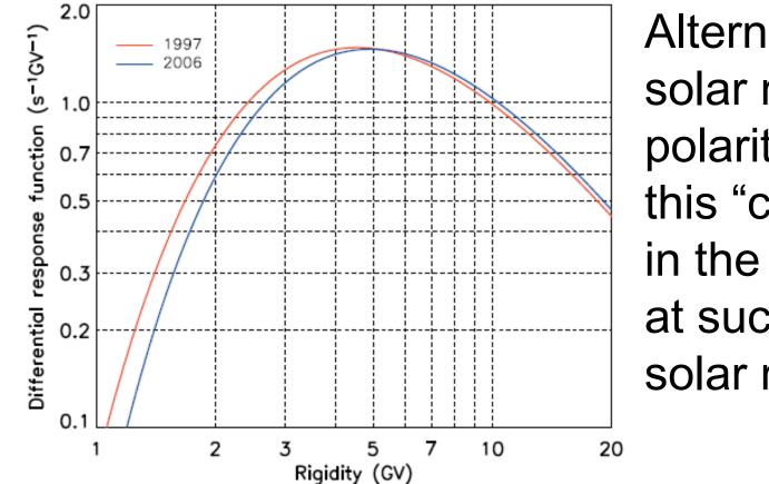
Alternating solar magnetic polarity creates this "crossover" in the spectrum at successive solar minima
