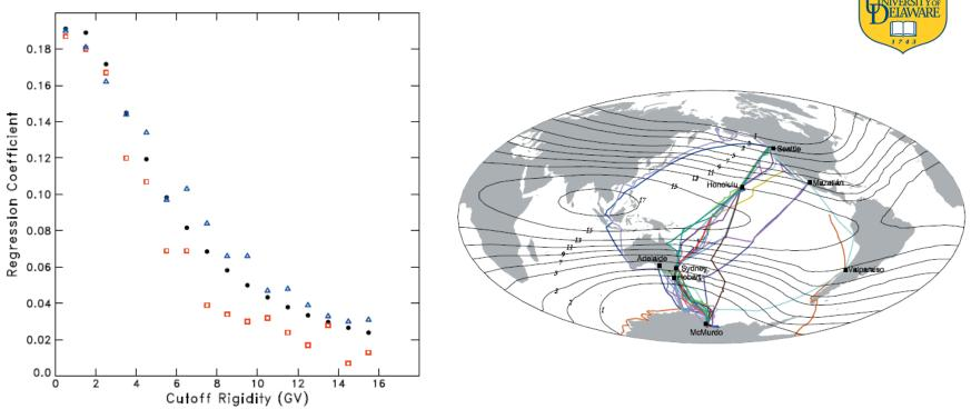
Regression analysis of a series of ship borne latitude surveys tracks the evolution of the spectral crossover in opposite solar magnetic polarity epochs.
