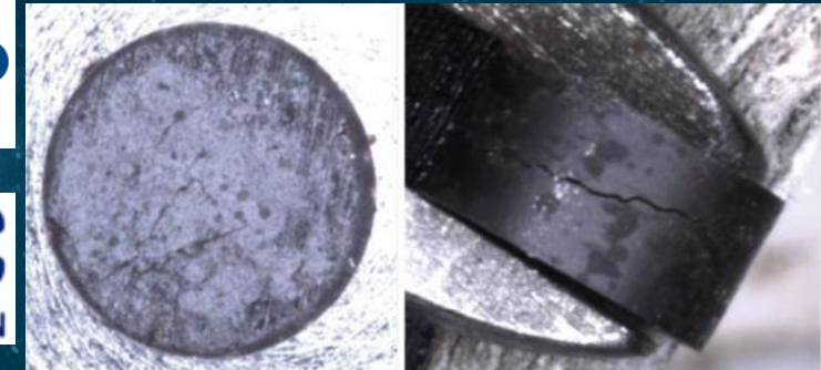
Experimental \text{Am}_2\text{O}_3 pellet
