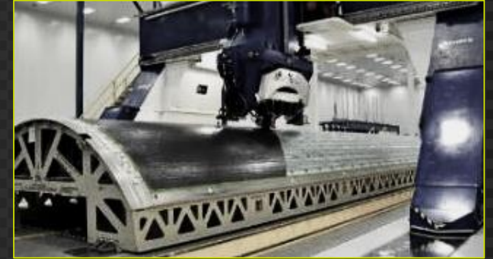
Robotic Composites Production (AFP) Superior 21 st century structural materials /manufacturing methods
