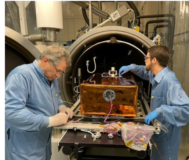
Preparation for Thermal-Vacuum Testing 03/08/2022
