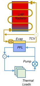
Pumped fluid loops (PFL) have a long heritage of use in human rated systems. They can collect large amounts of waste heat and transport it over long
