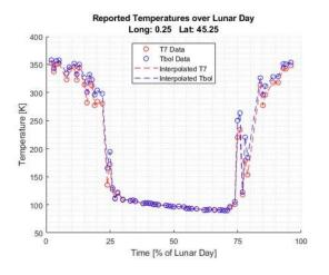
**Developments:** Marshall Space Flight Center (MSFC) has been a leader in developing thermal control systems for surviving in the extreme thermal environments of the Moon. In coordination with partners such as Advanced Cooling Technologies (ACT) and Masten Space Systems, MSFC has been testing several thermal control devices that can be used to help solve the problem of surviving in extreme Lunar environments.
