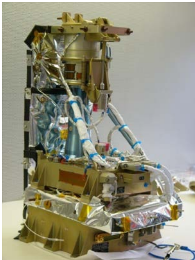
Fig. 1: Dawn FC without MLI (Sierks et al. 2011).
