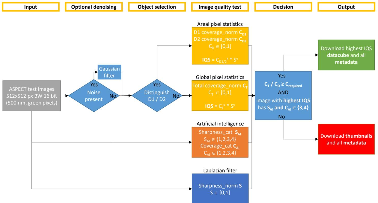
Fig. 1. On-board image quality detection algorithm architecture.
