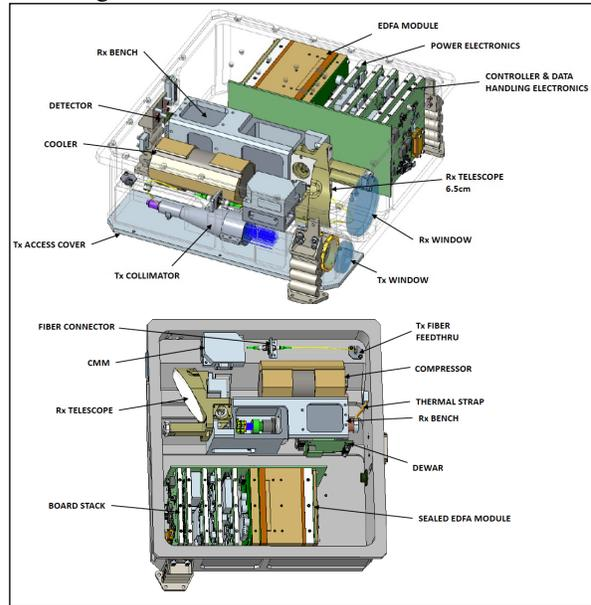
Figure 1. Small All-Range Lidar (SALi).
