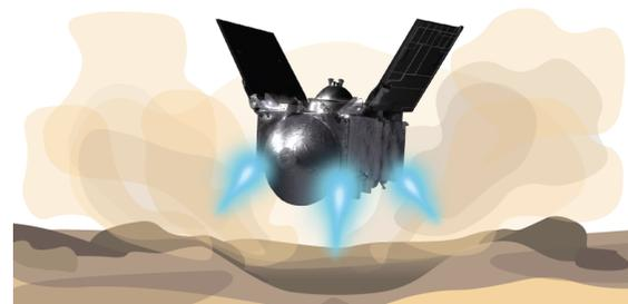
**Figure 1.** The REST maneuver shown in this cartoon will use the spacecraft’s thrusters to mobilize surface material, providing insight into the near-surface properties of Apophis.
