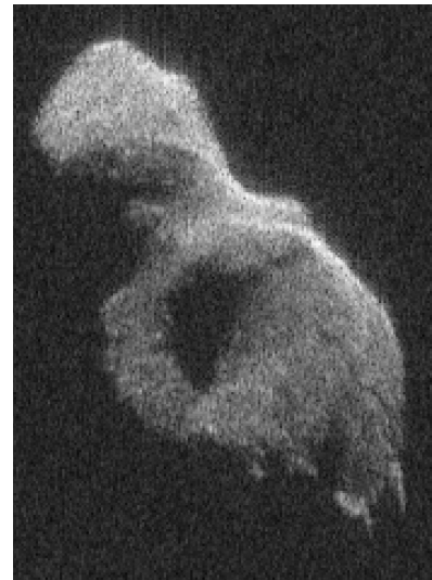
Figure 2. Delay-Doppler image of 2014 HQ124, an object similar in size to Apophis, obtained in 2014 using DSS-13 to transmit and Arecibo to receive. The range resolution is 3.75 m/pixel. Goldstone images of Apophis in 2029 should achieve a resolution of 1.875 m/pixel and reveal even more detail than is evident on 2014 HQ124.
