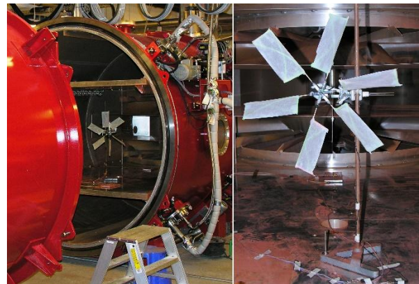
Figure 1: (left) The wind turbine positioned in the wind tunnel, which is 2 m in diameter. (right) Close-up of the wind turbine, with the wind tunnel fan visible in the background.
