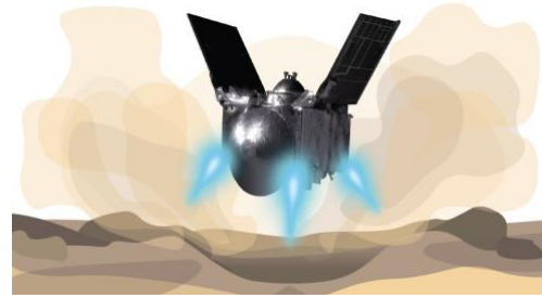
Figure 1. The STIR maneuver shown in this cartoon will use the spacecraft’s thrusters to mobilize surface material, providing insight into the near-surface properties of Apophis.
