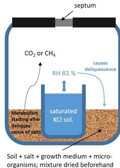
Figure 1: Experimental setup for investigation of metabolism rates of halophilic microorganisms in soil/salt samples that provide water by deliquescence only.
