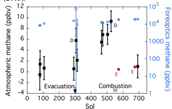
Redraft of Fig. 1, Webster et al [9]. "D" are daytime measurements, "E" enrichment. Foreoptics CH<sub>4</sub> – FL air before evacuation, rover sources thereafter – computed from table S2 in SOM [9].
