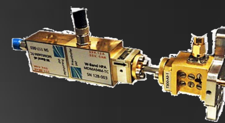
Figure 4. 17 cm X 3 cm 557 GHz receiver for space applications (TeraComp).
