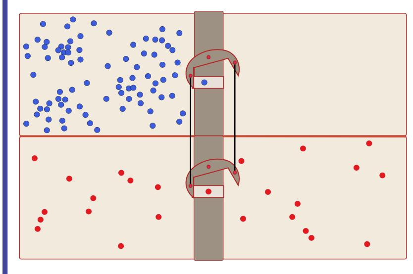
• Starting state: full disequilibrium in blue; approximated equilibrium in red. Particles and escapement motions driven by thermal fluctuations.
