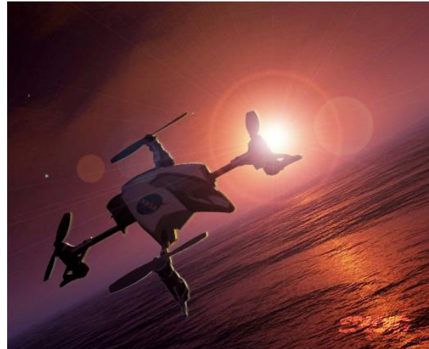
Figure 3 Concept for a Titan rotorcraft flying over a Titan lake. The vehicle is powered with a rechargeable battery and must return to a mother craft to recharge.
