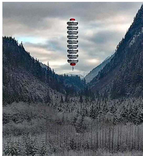
Figure 1 Mechanical Compression Altitude Control balloon is comprised of a number of segments that are compressed by shortening a tether that runs down the axis of the balloon. Release of the tether allows the balloon to rapidly ascend
