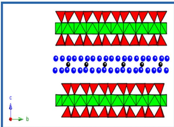
**Fig. 5 Mineral structure of smectite clays.** This diagram illustrates the water molecules (blue) and Na/Ca cations (black) in the interlayer region (blue), metal cations in the octahedral layer (red), and Si in the tetrahedral layer (green) [18].
