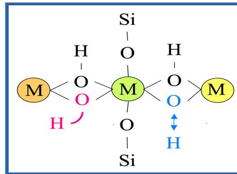
**Fig. 6 OH bonds in phyllosilicate structures.** This diagram illustrates the bonding configuration of the octahedral layer [from 18]. The OH stretching (blue) and bending (pink) motions have vibrational energies that depend on the type of metal cations (M) occupying the octahedral sites in the mineral structure.
